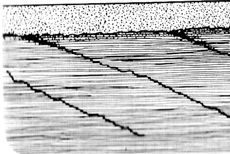
Figure 1(c) Fissure development in mudstone/ shale/ coal measures
